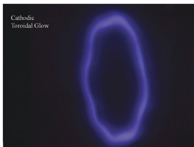
Figure 7 Pictorial view of the toroidal glow develops by a magnetic field enhanced electrode by audio frequency discharge. The toroidal glow develops near the surface where the magnetic field line is parallel to the electrode surface. The glow develops only in the toroidal glow and the remaining surface of electrode is not participating with the creation of luminous gas phase. [Color figure can be viewed in the online issue, which is available at wileyonlinelibrary.com .]
