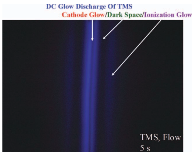
Figure 2 The glow develops at the onset of gas phase breakdown of TMS. The main glow is the dissociation glow of trimethylsilane touching to the cathode surface; i.e., there is no cathode dark space. The second glow (ionization glow), which develops subsequent to the dissociation glow, is separated from the cathode surface as well as from the dissociation glow by the cathode fall. [Color figure can be viewed in the online issue, which is available at wileyonlinelibrary.com .]
